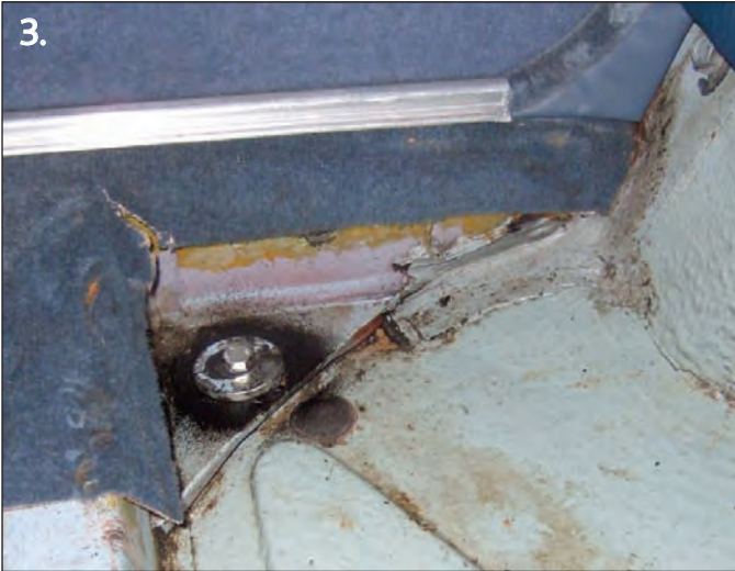
3. (Photo 3). The top spring mounts on the rear box sections can also weaken, so check here and for an unequal ride height.
